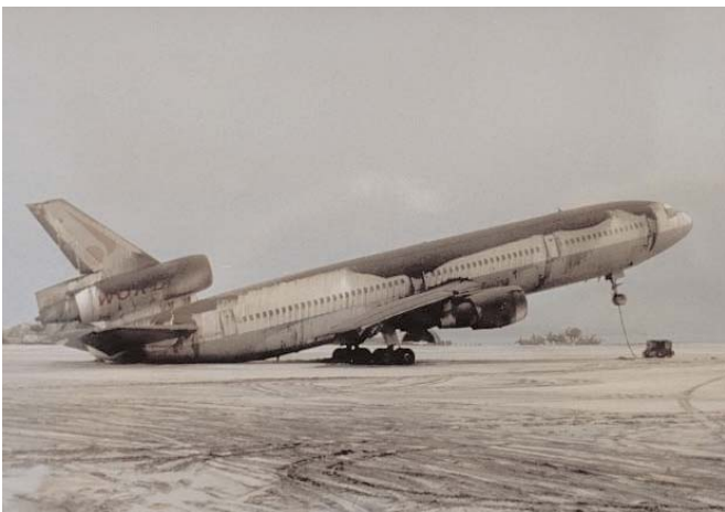
Figure 2. Heavy ashfall from the 1991 eruption of the Pinatubo volcano in the Philippines caused this World Airways DC-10 to set on its tail. About 4 cu km of ash was erupted on 15 June. It accumulated to depths of 10-15 cm at this airfield at the Cubi Point Naval Air Station, 40 km SSW of Pinatubo. [Photo: R.L. Rieger, U.S. Navy]
