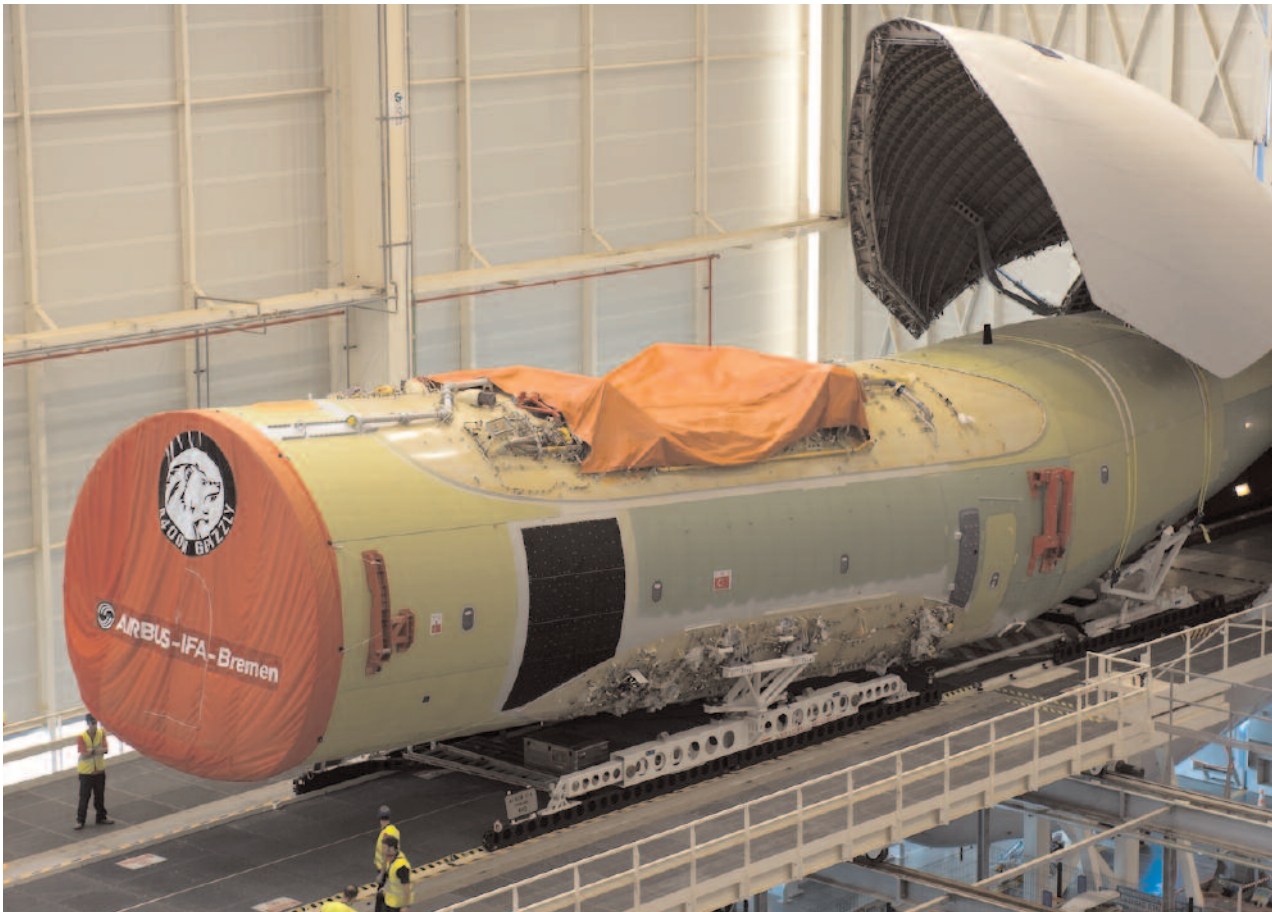
Figure 3: Manufacturing of the nose and of the fuselage in Bremen. Credit: Airbus Military
