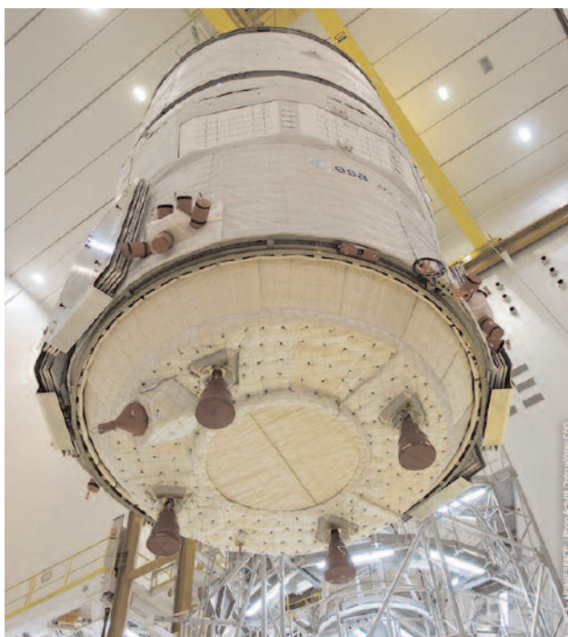
Figure 3. Service Module being hosted for mating with the ICC. Credit ESA
