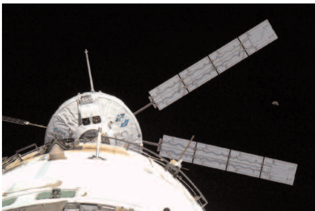
Figure 1. ATV remains attached as a pressurised module and integral part of the ISS for up to 6 months.
