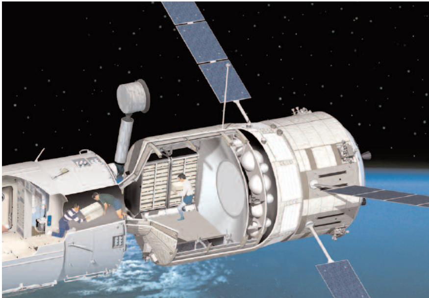
Figure 4. Powered by the ATV Service module, the Integrated Cargo Carrier (ICC) is the core room of the ATV, it makes up 60% of ATV's total volume. Its maximum capacity is 6.6 tonnes of cargo. Credit ESA
