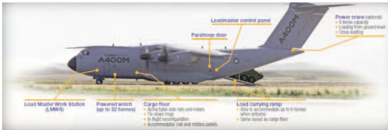
Figure 9. Autonomous ground operations: once the A400M on the ground, a rapid and autonomous cargo loading or unloading can be performed without any specialized ground support equipment.
