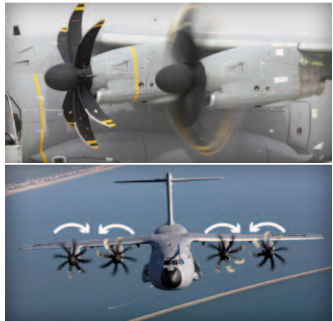
Figure 3. The down between the engines counter-rotation of the propellers, which turn in opposite directions, allows a structural weight reduction.
