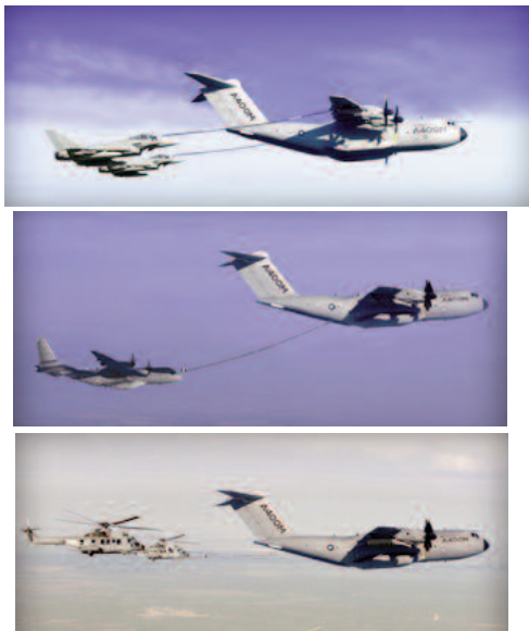
Figure 10. The A400M is the only tanker which can refuel the entire range of probe-equipped military aircraft or helicopter at their preferred speeds and altitudes.
