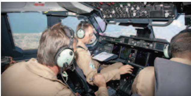
Figure 4. State-of-the-Art cockpit: the A400M features 2 HUDs which provide the pilots with all primary flight information together with flight director orders and flight guidance during critical mission phases; it also features 8 large interchangeable liquid crystal head-down displays.
