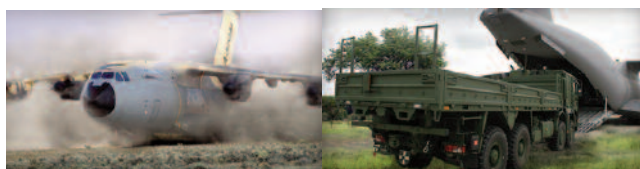
Figure 8. The A400M is able to land on and take-off from any short, soft and unprepared airstrip no longer than 750 m.
