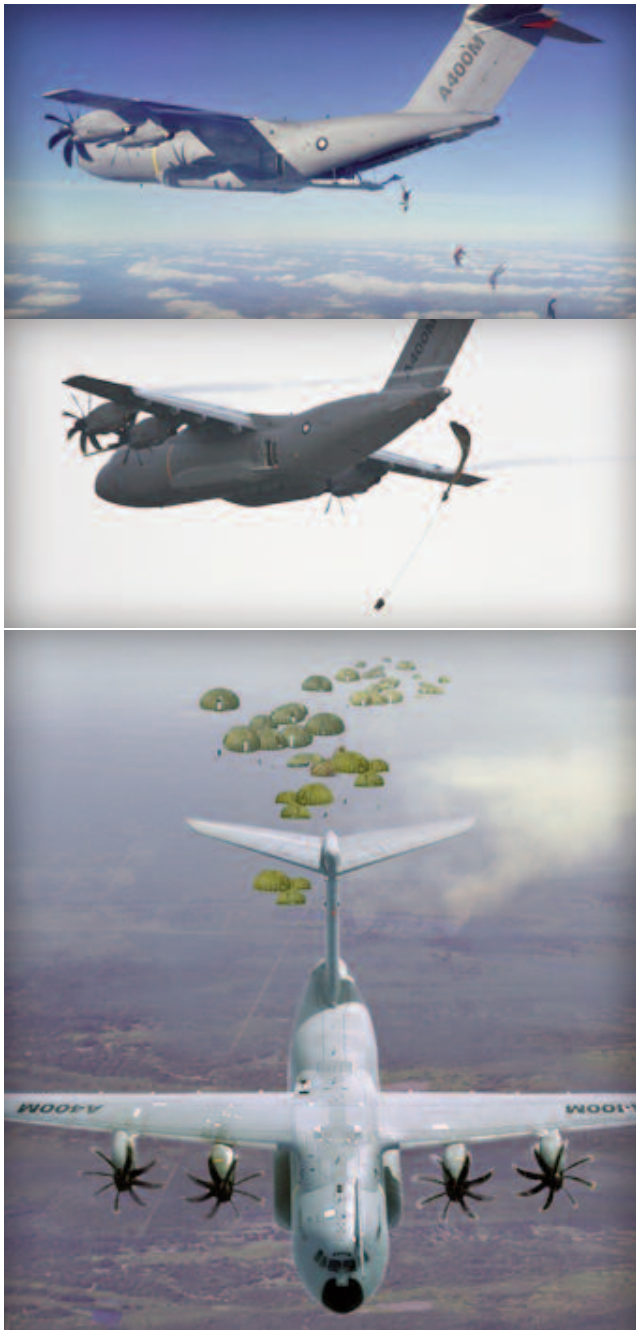
Figure 6. The A400M can accommodate up to 116 fully equipped paratroopers, carrying them to the DZ (Dropping Zone) at speeds up to 300 kt, but dropping them at as little as 110 kt to ensure minimum dispersion.
