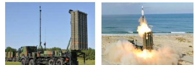
Figures 8.3 and 8.4: The Launching Modules armed with 8 hyper-velocity Aster missiles, « The sword».
