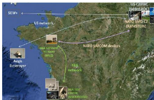
Figure 5: The architecture of the missile defense during the live firing, from bottom to top. The Franco-Italian crew operated 2 SAMP/T sections and intercepted a ballistic target, representative of a SCUD type short range missile. The designation of the SAMP/T was done by a local radar situated in Biscarrosse via a L16 datalink. The chain of command consisted of a French C2 center at Bruz which assured the interface with the command center in Ramstein, regrouping the NATO BMDOC with the ACCS system and the US C2BMC command center, linked with an American Aegis destroyer.
