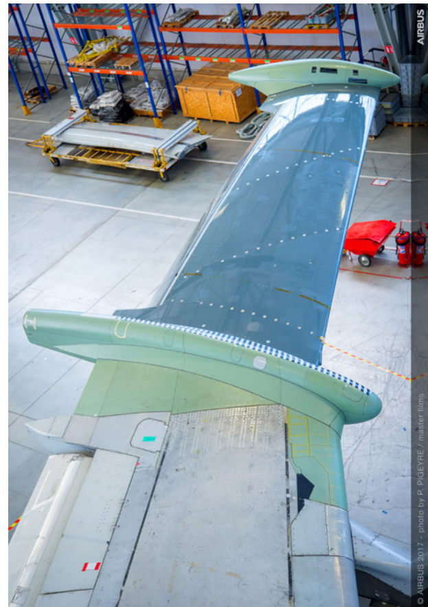
The smooth surface of the BLADE aircraft's outer wing section. Source: Airbus Airbus photo blade wing P.Pigeyre/Master Films the laminar wing based on Bjorn's Corner: Laminar flo
