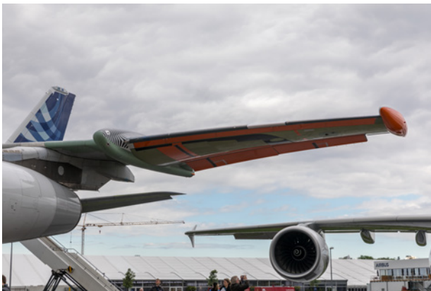
The left laminar flow wing section
