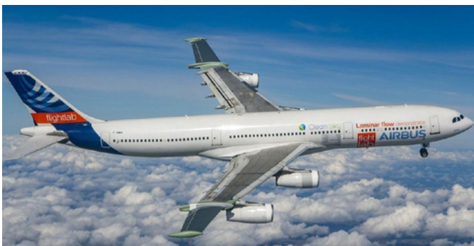
Fig. 5: The Airbus A340-001 with modified outer wings for the laminar flow flight tests of Clean Sky in 2018 (©Airbus)
