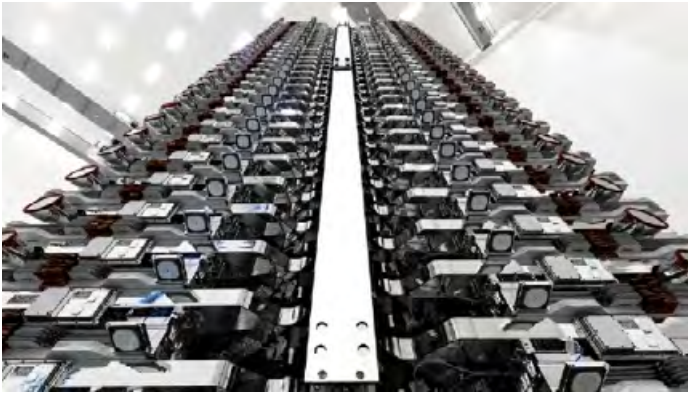
Figure 3: New Space approach example: 60 Standardized Starlink satellites loaded in one Falcon9 launcher (www.Starlink.com)
