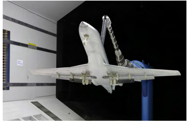
Swiss aeronautical innovation: In RUAG's wind tunnel, the aerodynamics of new aircraft and aircraft concepts are investigated using the latest measurement methods; the picture shows the Swiss Pilatus PC-24 business jet. (Image: RUAG)
